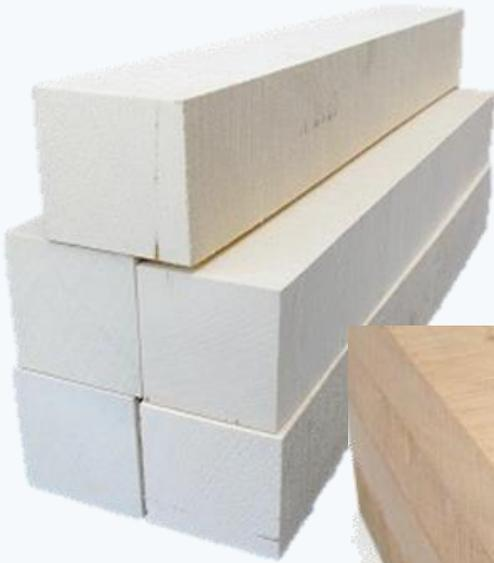
Holly is hard, has no discernable grain, and can have visible growth rings. It's color can run from pure white, to shades of cream, and sometimes gray. It all depends on how it was cut and seasoned. It carves well, it bends even better, just use heat or steam. It is also used for decking.
