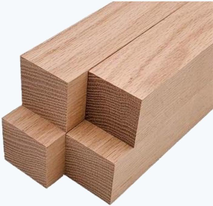
Oak should not be used in your ship model under any circumstances. Use it for the case and base, and that is all. Notice the very pronounced grain and growth rings. Imagine scaling down this wood for use in your model. Now imagine the wood pores, which didn't scale down, becoming 2, 3 4, 5 inches in scale cross-section.
