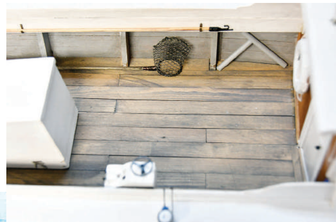
The deck boards were milled by model builder Don Good and stained to give them a worn look. Note the boat hook and net.
